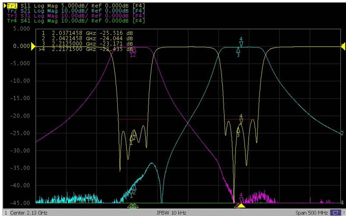
A third harmonic rejection requirement meant that a notch was needed which was realised using specially placed tuners. The same basic housing is used for the two filters or diplexer. The only difference being the number of output connectors.
